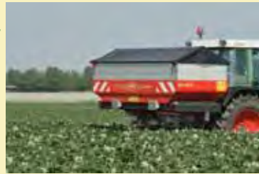
Double overlap spread pattern. Spread widths up to 148' Capacities up to 8200#.
